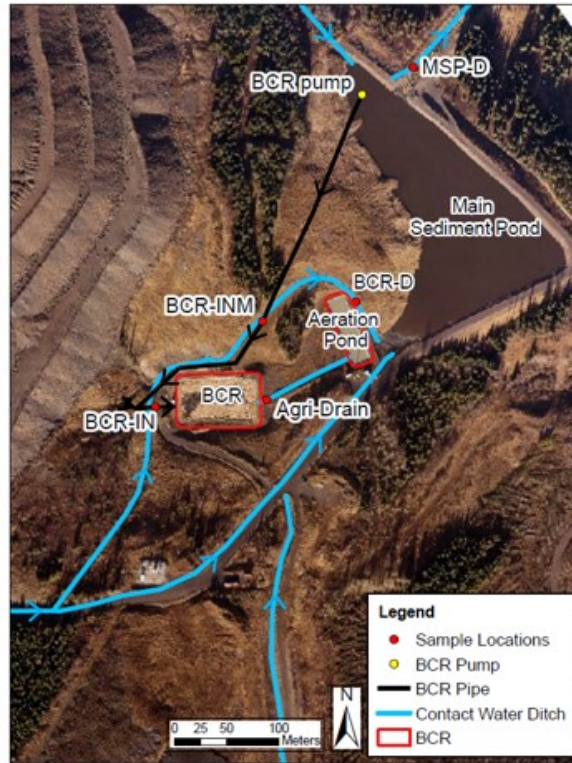
Figure 3. Sampling Locations for Monitoring the Efficacy of the BCR System at the Brule Mine.
